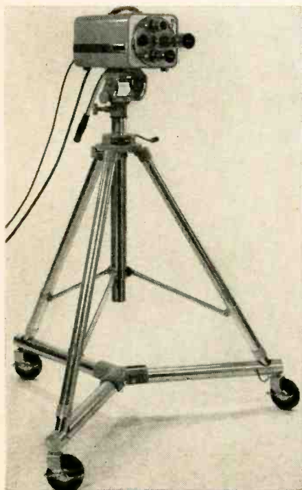
Argus CCTV camera on its mobile tripod.
